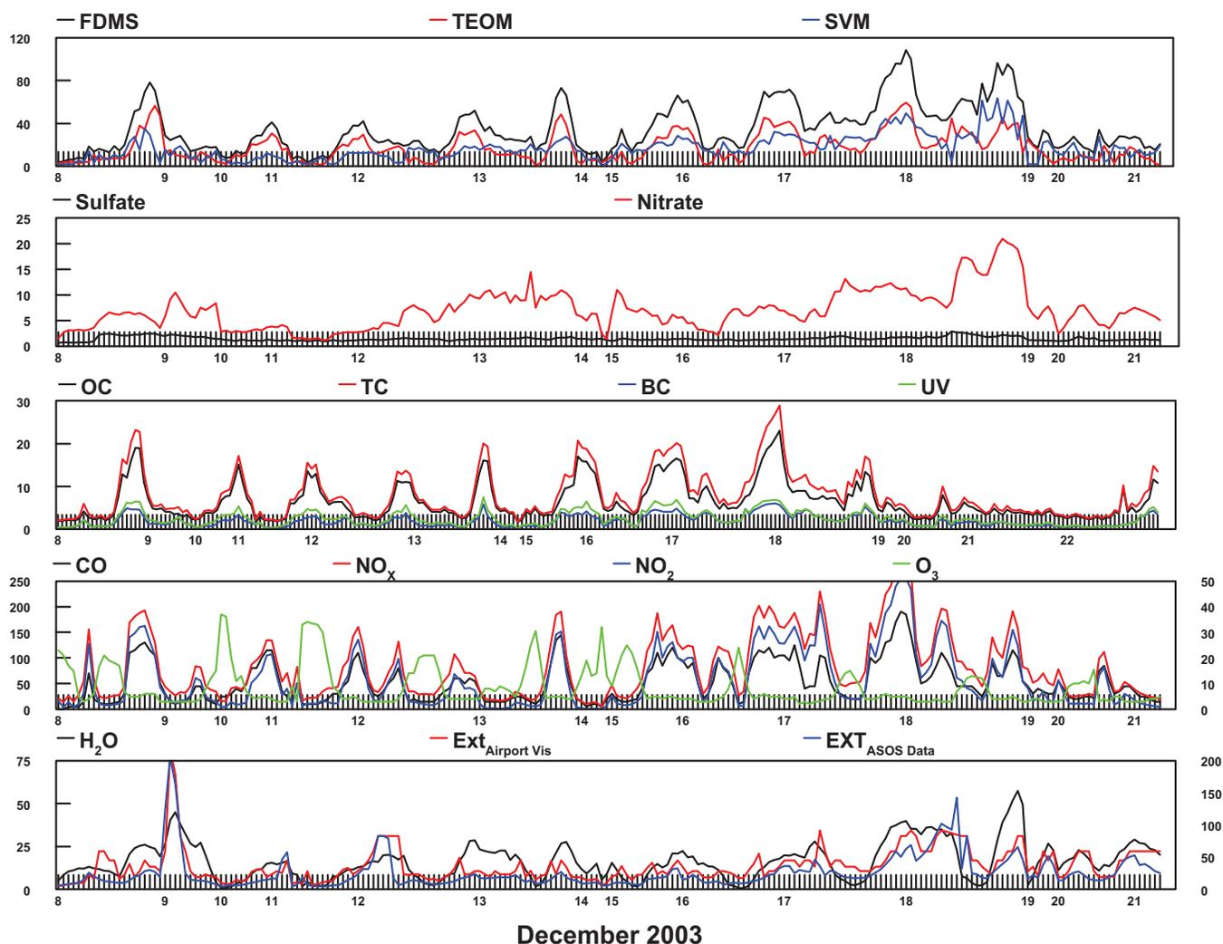
**Figure 6.** Concentrations of the various species used in the PMF analyses for the Fresno 2003 study. The data in the bottom chart were used for the PMF with extinction analysis. The other data were used in conventional PMF and PMF with extinction analyses. Units for all particulate components are  $\mu\text{g}/\text{m}^3$ . Units are parts per million (ppm) for CO and parts per billion (ppb) for the other gases. Units for both extinction values are  $\text{Mm}^{-1}$ .
