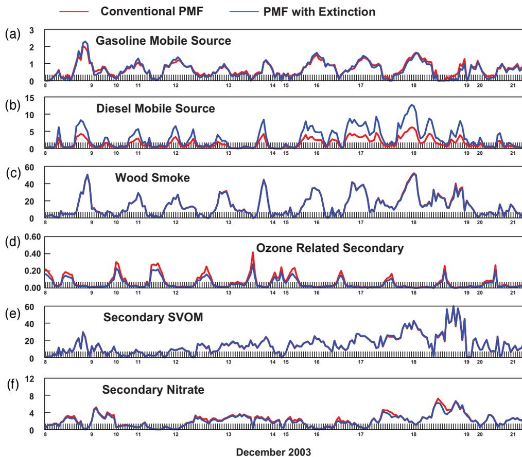
**Figure 10.** 2003 Fresno  $PM_{2.5}$  data for the identified six sources of the conventional PMF and PMF with extinction. Comparing the two analyses, the diurnal patterns associated with each source are similar and, except for the diesel mobile source, concentrations are similar. Sources include (a) gasoline mobile, (b) diesel mobile, (c) wood smoke, (d) ozone-related secondary, (e) secondary SVOM, and (f) secondary nitrate.
