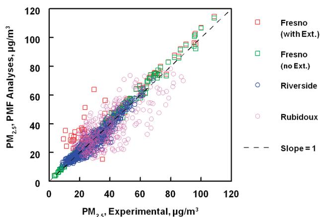
**Figure 9.** Experimental  $PM_{2.5}$  mass compared with the calculated sum of the  $PM_{2.5}$ . All factors for the various PMF with extinction analyses and the conventional PMF analysis at Fresno are plotted. The linear regression results for the fit of the various datasets are found in Table 1. The greater scatter in the data for the Rubidoux site is due to increased uncertainty in the low-resolution extinction data for this site.
