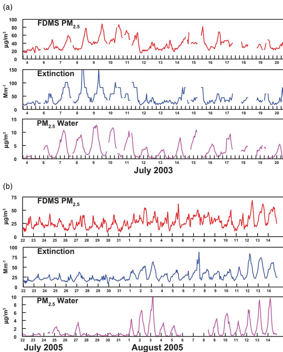
**Figure 7.**  $PM_{2.5}$  extinction and PM water used in the PMF with extinction analysis. (a)  $PM_{2.5}$  extinction for Rubidoux 2003 and (b) for Riverside 2005.
