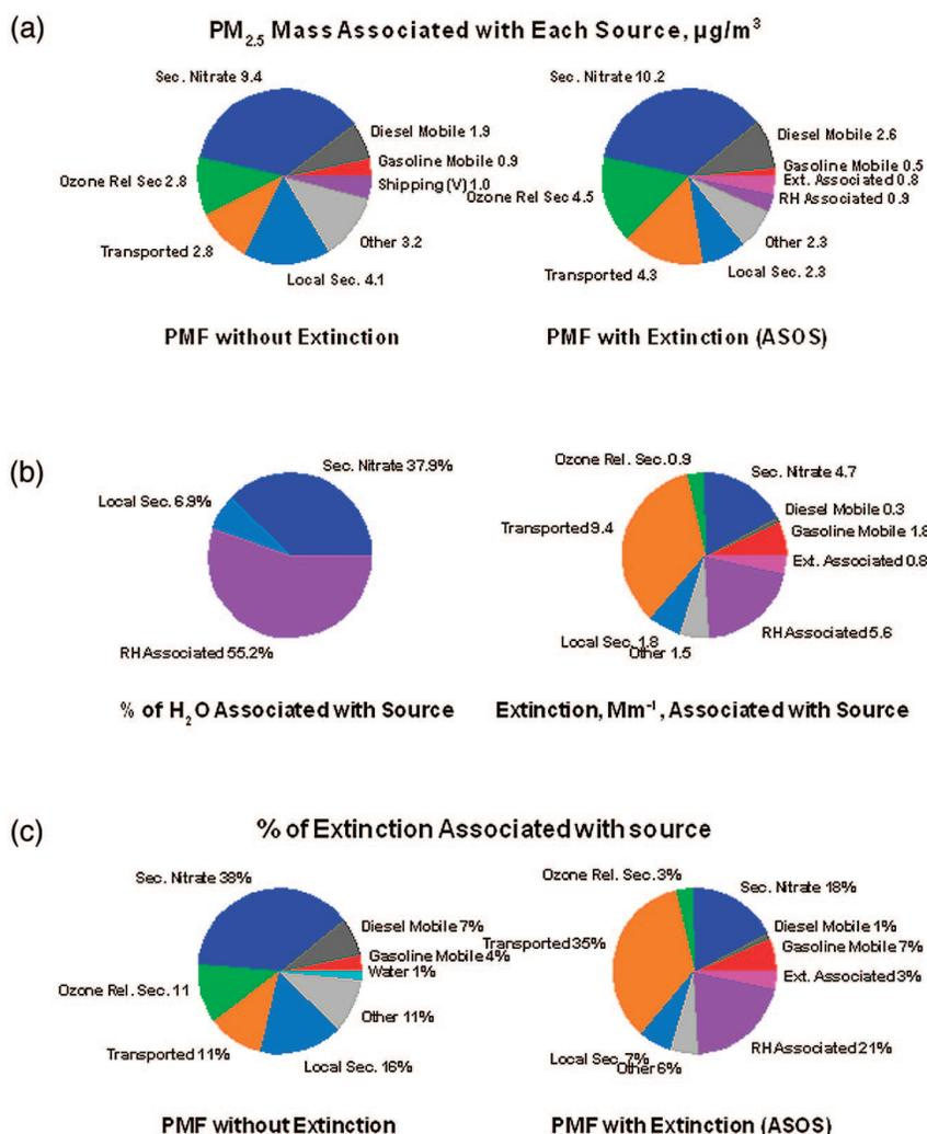
**Figure 17.** Pie charts comparisons using the Riverside 2005 data. Chart (a) shows the PM<sub>2.5</sub> mass associated with each source identified in the PMF with extinction and PMF without extinction analyses. Chart (b) shows the percentage of modeled particulate water and Mm<sup>-1</sup> of extinction associated with each factor for the PMF with extinction. Chart (c) shows the percentage of extinction associated with each source for the PMF without extinction and PMF with extinction.
