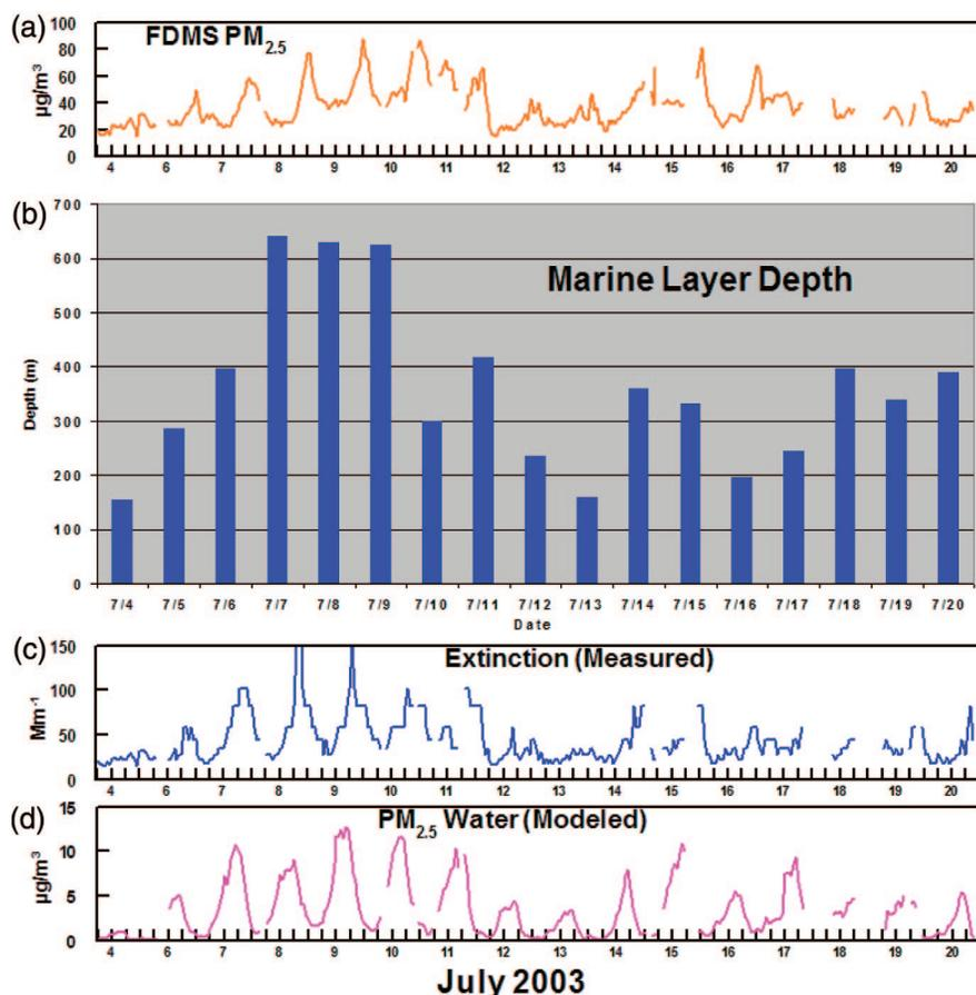
**Figure 15.** Four temporal graphs from July 4 to July 20, 2003 at Rubidoux. The graphs include (a) the FDMS  $PM_{2.5}$ , (b) marine layer depth, (c) the measured extinction converted from Riverside Municipal Airport ASOS hourly averaged visibility, and (d) the modeled  $PM_{2.5}$  water associated with sulfate and nitrate aerosols. Note that when the marine layer deepened from July 7 to 9, the  $PM_{2.5}$  mass, extinction, and modeled water also increased.
