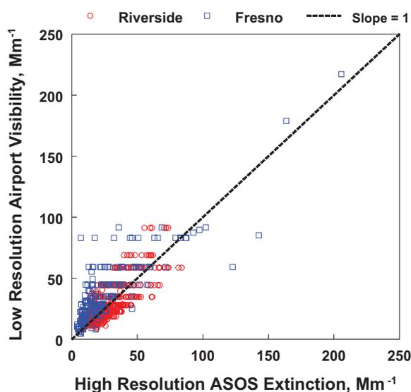
**Figure 8.** Comparison of high-resolution ASOS and low-resolution extinction data from the Riverside and Fresno airports. The low-resolution data originated from the airport visual range data. These data are given in mile increments, accounting for the layered nature of the comparison at higher extinction values.
