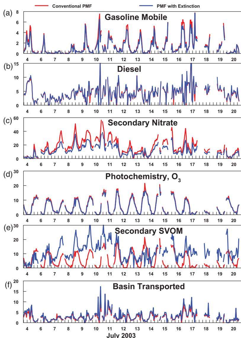
**Figure 1.** 2003 Rubidoux  $PM_{2.5}$  data for conventional PMF and PMF with extinction. The diurnal patterns associated with each identified source are similar for the two analyses. Source concentrations are also similar except for secondary nitrate and secondary SVOM. Sources include (a) gasoline mobile, (b) diesel mobile, (c) secondary nitrate, (d) photochemistry,  $O_3$  (e) secondary SVOM, and (f) basin-transported.
